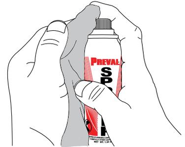
If spraying thicker latex paint, hold a rag over the red insert in the button and push the button down for three seconds. You will see bubbles in the liquid as the paint is returned to the container. This will lubricate the passages in the power unit and allow smooth paint flow through the nozzle.
